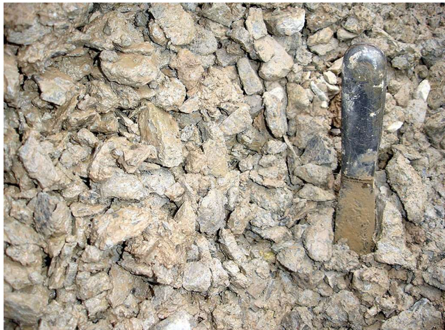
Figure 5: Crushed Rock After Migration of Backfill Soil
