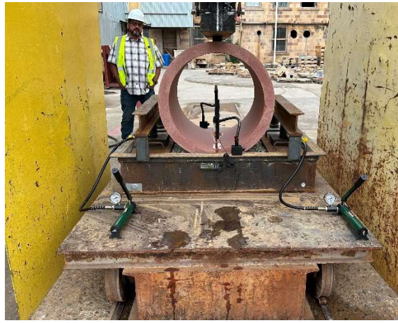
Figure 9: Test Set-Up with 24-inch diameter pipe and soil box
