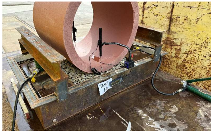
Figure 10: Surcharge Loading with Steel Plates/ Hydraulic Jacks on the Bedding Soil
